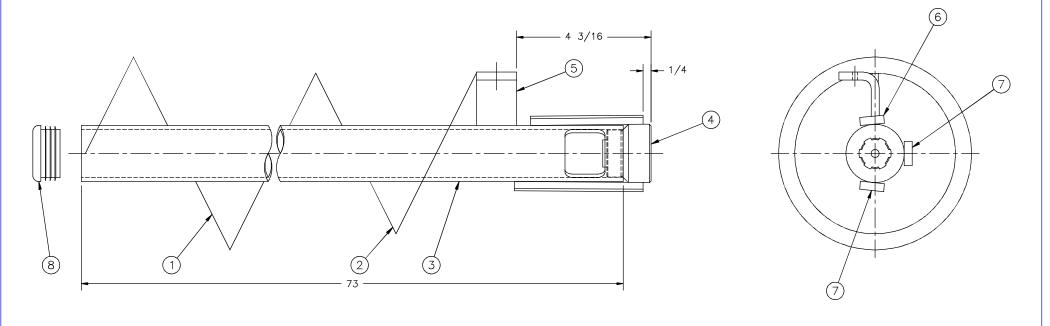
THIS AUGER ASSEMBLY IS USED ON HYDRA FEEDERS WITH SENSOR AND MAGNET.
